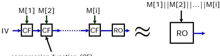
compression function (CF): Hirose, Tandem-DM, Abreast-DM
